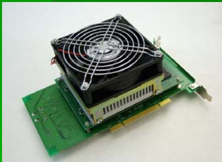
Fig 1: A single GRAPE-6A card fits into the PCI-slot of a common PC and can accelerate the force calculation in an N -body simulation by a factor of 100. The peak-performance is 125GFlops but the card's memory can only hold 128k particles.
