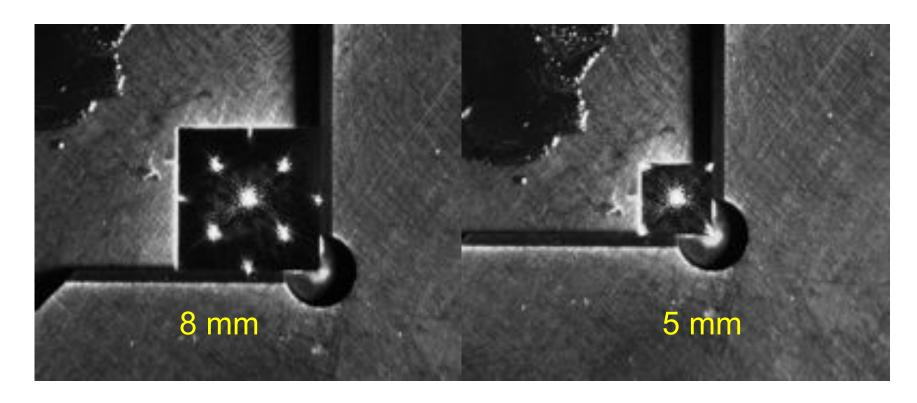
Spatial filter blades block DM waffle (0.5 µm) & scalloping, eliminating aliasing in the wavefront sensor
