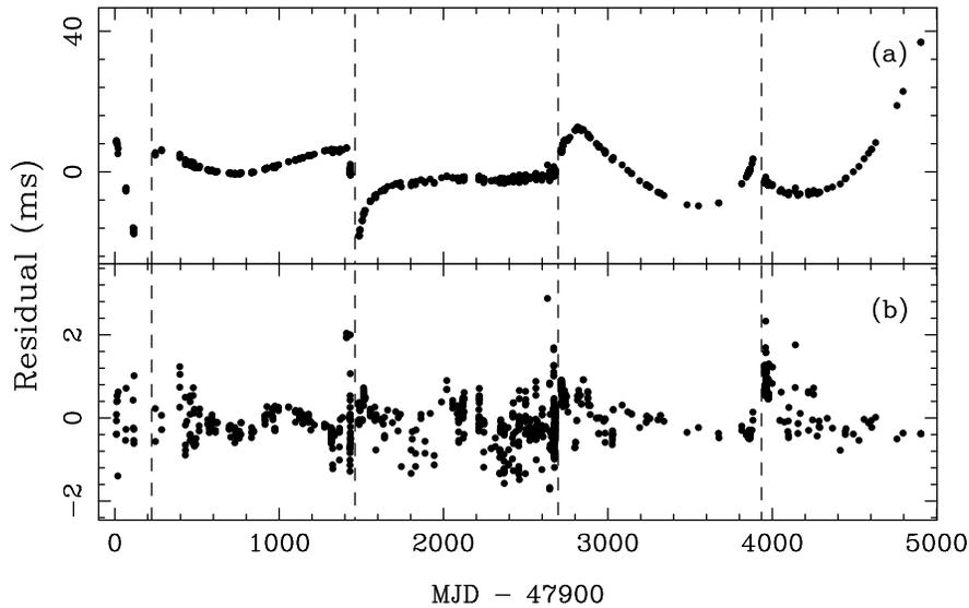
Figure 1. Residuals as a function of time for the entire 13-year data set on PSR B1259–63. The top panel shows the residuals after fitting for spin-orbit coupling terms. The bottom panel shows the best fit we obtained, which includes jumps in  $x$  at each periastron.
